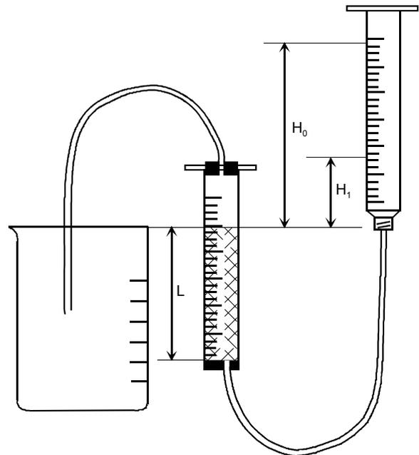
**Fig 2.** Application of the syringe minipermeameters in a falling head test. Measurements and calculations are described in the text.
