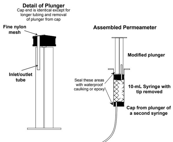
**Fig. 1.** Construction of the syringe minipermeameters. Dimensions and materials are given in the text.
