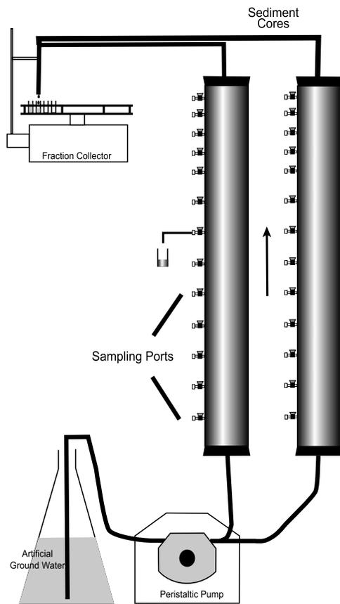
**Figure 1.** Schematic diagram of the laboratory column setup. A peristaltic pump was used to pump AGW into the intact cores from the bottom. Pore water samples were collected through the sampling ports. An automatic fraction collector was used for continuous sampling of effluent.
