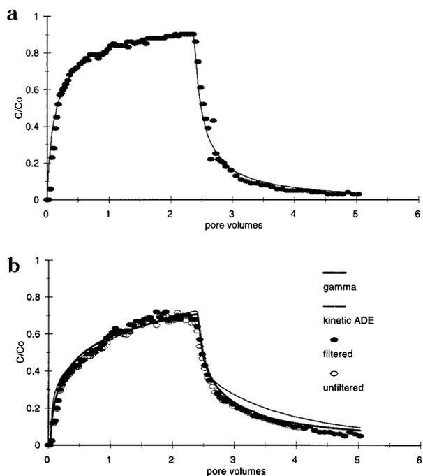
**FIGURE 2. (a) Breakthrough curve of <sup>3</sup>H<sub>2</sub>O and calculated ADE model fit for -19 cm experiment. (b) Hydroxyatrazine breakthrough (filtered and unfiltered) for -19 cm experiment and calculated curves for the kinetic ADE and  $\gamma$ -distributed desorption (gamma) models.**
