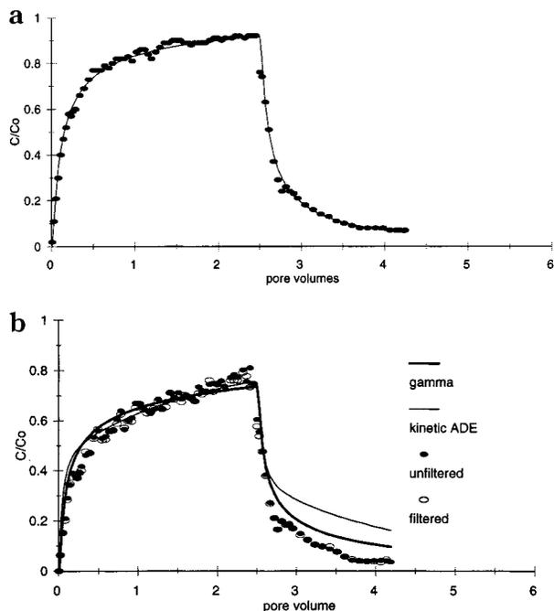
**FIGURE 1. (a) Breakthrough curve of <sup>3</sup>H<sub>2</sub>O and calculated ADE model fit for -8 cm experiment. (b) Hydroxyatrazine breakthrough (filtered and unfiltered) for -8 cm experiment and calculated curves for the kinetic ADE and  $\gamma$ -distributed desorption (gamma) models.**
