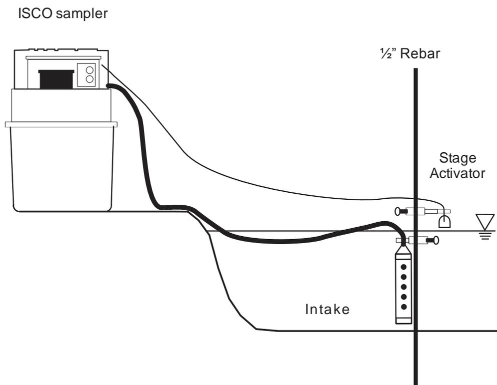
Fig 2.2 Schematic of the stage-activated automatic sampler for collecting stream water at regular intervals during storms.
