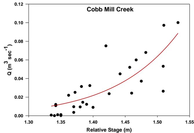
**Figure 2.3.** Rating curve for the culvert gauge at Cobb Mill Creek. (Pickus *et al.*, 2014)
