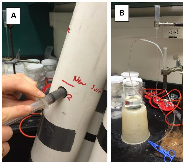
Figure 1: Sample collection from sediments cores. A: A subcore is extracted in a detipped syringe. B: The mini-permeameter setup includes a syringe falling head tank, the subcore, and a beaker for base level.
